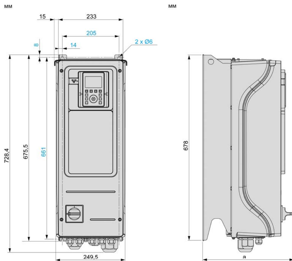
ATV950U07N4E, U15N4E, U22N4E, U30N4E, U40N4E, U55N4E:  $a = 300$  мм
