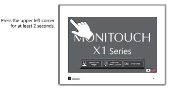
2. Then within one second, press a different corner and hold for at least 2 seconds to display the status bar.
