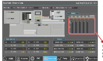
The  $\triangle$  icon appears at the top right corner of the part that monitors the device memory of a device in which a time-out error was detected.
