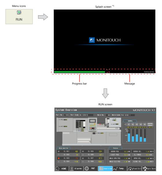
\*1 The splash screen can be changed as desired. For details, refer to the X1 Series Reference Manual 2.
