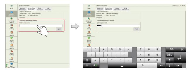
2. Press the [Apply] switch. The following confirmation dialog appears. Press the [OK] switch. All items that were prohibited in Local mode become unprotected.
