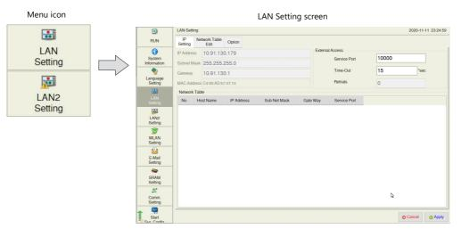
When no LAN cable is connected or a link is not established, the indication of the [LAN Setting]/[LAN2 Setting] icon is changed as follows.
