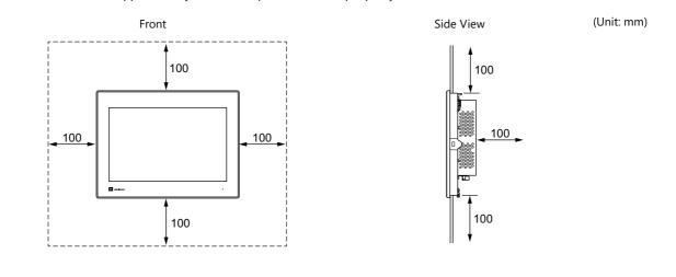
Mount the X1 series unit with approximately 100 mm of space around the periphery of the unit.
