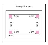
2. Then within one second, press a different corner <sup>\*1</sup> and hold for at least 2 seconds to display the system menu.
