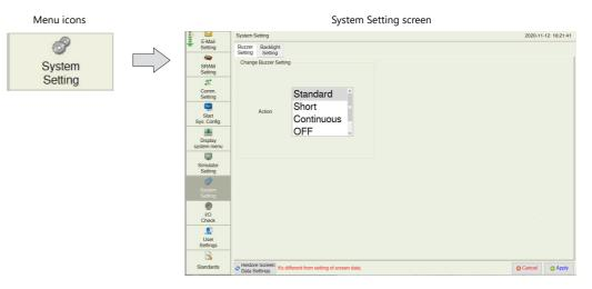
System Setting 2020-11-12 18:21:41 E-Mail Setting Buzzer Backlight Setting Setting SRAM Setting Change Buzzer Setting 2 Comm. Setting Standard Sys Short Action Start Sys. Config Continuous . OFF Display system me 510 Simulator Setting ð VO Check User Settings Press to revert to the Press the [Apply] switch to confirm the setting. 3 settings set in the tandards Hestore Screen Data Settings
