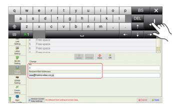
4. Press the [OK] switch and then the [Apply] switch. The changed address takes effect.
