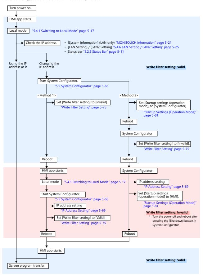
\*1 When [Write filter setting] is set to [Valid], some System Configurator settings cannot be changed. If a setting cannot be changed, set [Write filter setting] to [Invalid] and then change the intended setting. For details, refer to "Settings that Check the Write Filter Setting" page 5-79.
