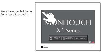
2. Then within one second, press a different corner and hold for at least 2 seconds to display the system menu.
