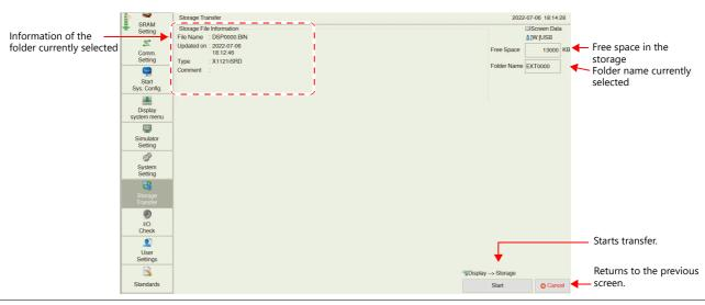
When selecting [Use Password When Transferring Screen to storage from Display] in [System Setting]  $\rightarrow$  [Other]  $\rightarrow$  [Storage Setting] using V-SFT version 6, the following screen is displayed before the screen explained in step 1 is displayed. Enter password, and press the [OK] switch.
