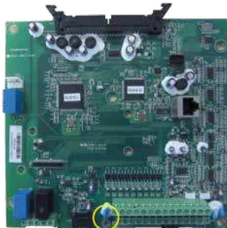
Disconnect the ground screw below the C/B and ground studs of isolated metal plate.
