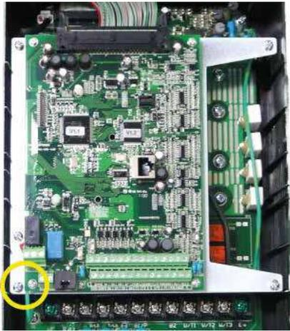
Disconnect the ground wire of isolated metal plate.
