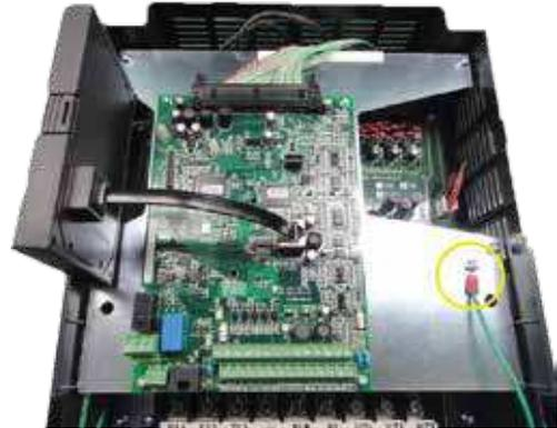
Disconnect the ground wire of isolated metal plate.
