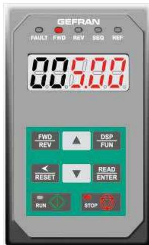
**Fig 5.2: LED Keypad (Running)**
