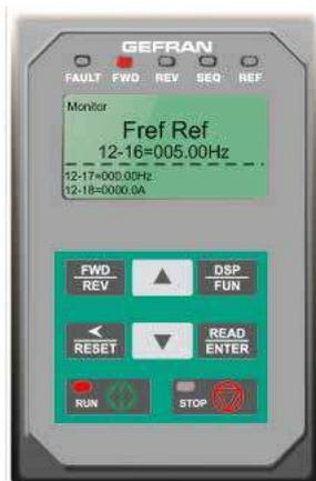
Use the **RUN** key to run the drive in forward direction and the FWD/REV key to change the motor direction. (Note: to disable reverse direction set parameter 11-01 to 1)
