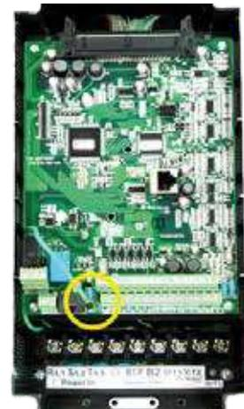
Disconnect the ground wire of J1. on the control board (C/B).
