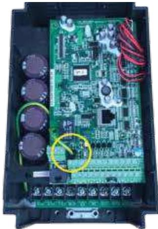
Disconnect the ground wire of J1. on the control board (C/B).
